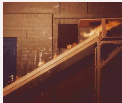
Flames attaching to a model of an escalator trench and jetting out of the top. [Fennell, 1988]
