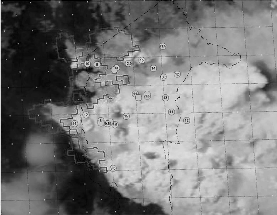
Figure 4. MODIS imagery of ACT and region, 14:00 18/1/03. This also shows a 10km grid (slightly skewed in this projection); the ACT border; automated fire mapping (by NOAA) and labelled circles showing inferred peaks of convection, with heights in km.
