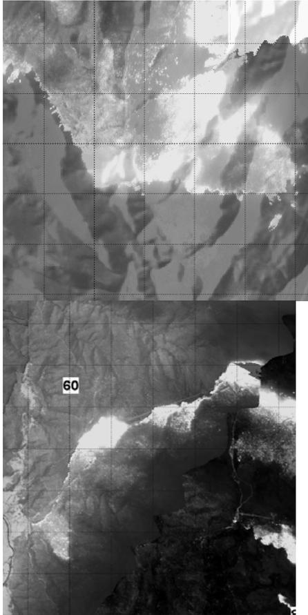
(B) Lee slope channelling, Glendale Depot, Stockyard Fire, 18/1/03. The lee slope of a NW-SE oriented ridge has caused the flank to deviate southwards by over 2 km. An additional terrain interaction is occurring on the downwind ridge, and cooler cores of at least 2 significant spotfires are visible.
